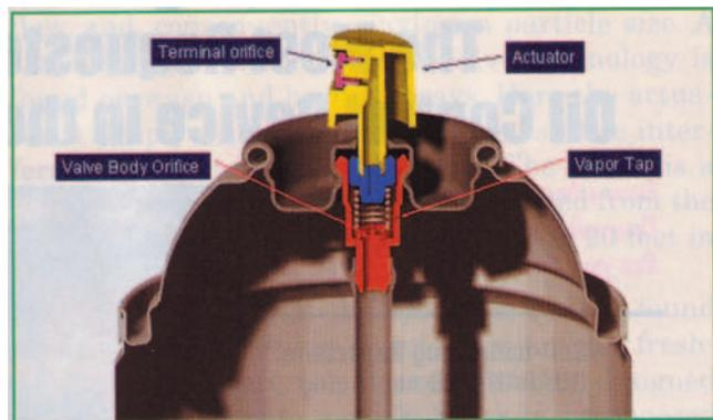
**Figure 4. Aerosol valve showing vapor tap location.**
