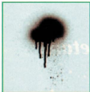
Figure 2. Coarse spray patterns with "hot spots."
